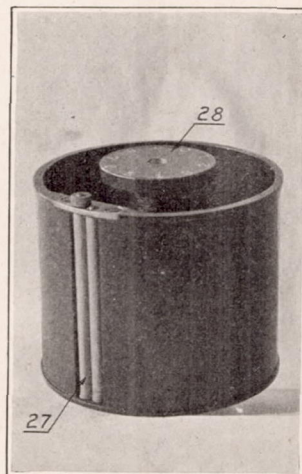
FIG. 6.—Film drum showing rollers for tightening film.
