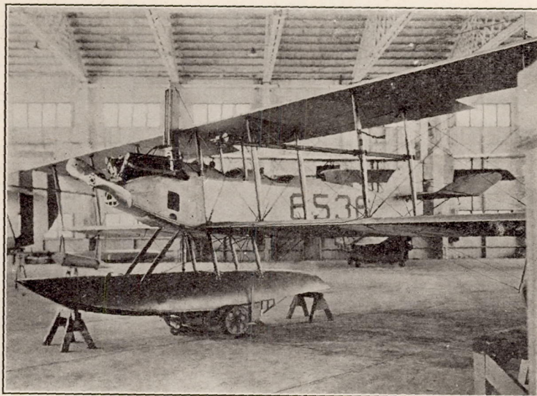
FIG. 2.—N-9H ready for planing test. Angle of attack controller vane in the foreground
