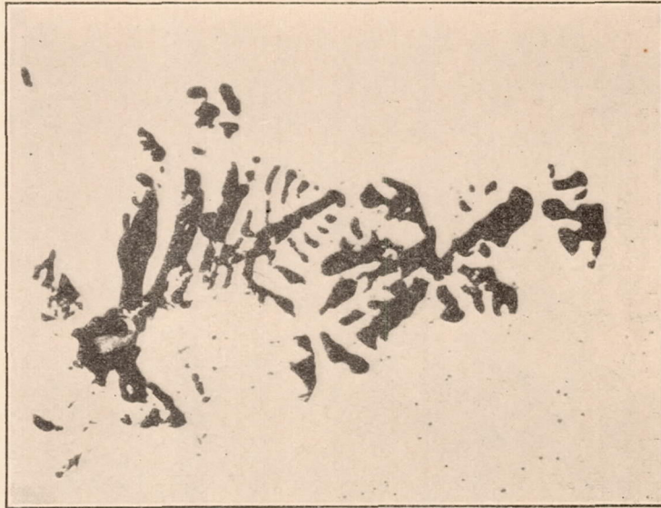
FIG. 9.—Mag. 100 X. Dendritic corrosion pits in magnesium-aluminum alloy after repolishing
