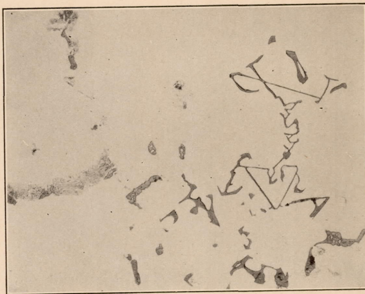
FIG. 15.—Mag. 200 \times . Microstructure of an alloy containing 5 per cent aluminum, 0.3 per cent silicon, balance magnesium
