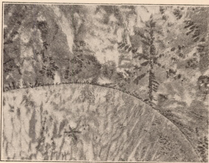
FIG. 18.—Mag. 50 X. Primary dendrite of magnesium in an alloy containing 3 per cent silicon. Note the identical form with corrosion pit of Figure 17
