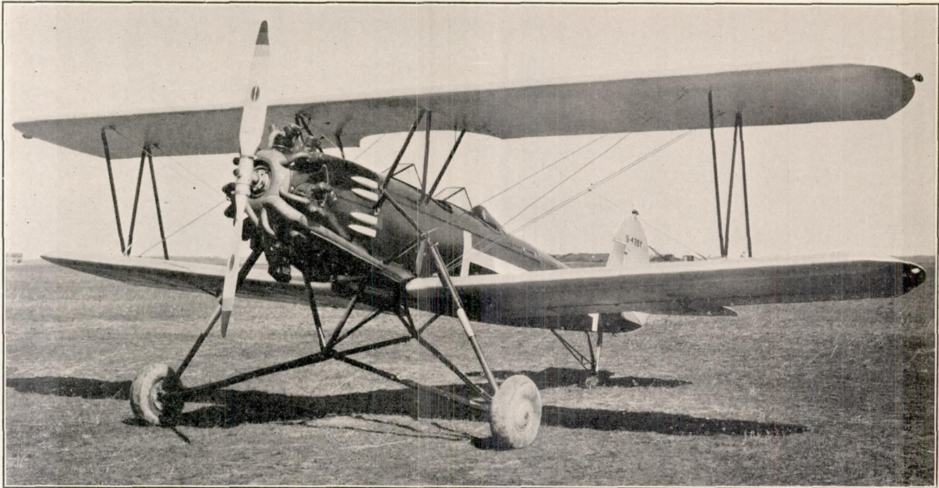
FIGURE 16.—Verville airplane modified for landing tests.
