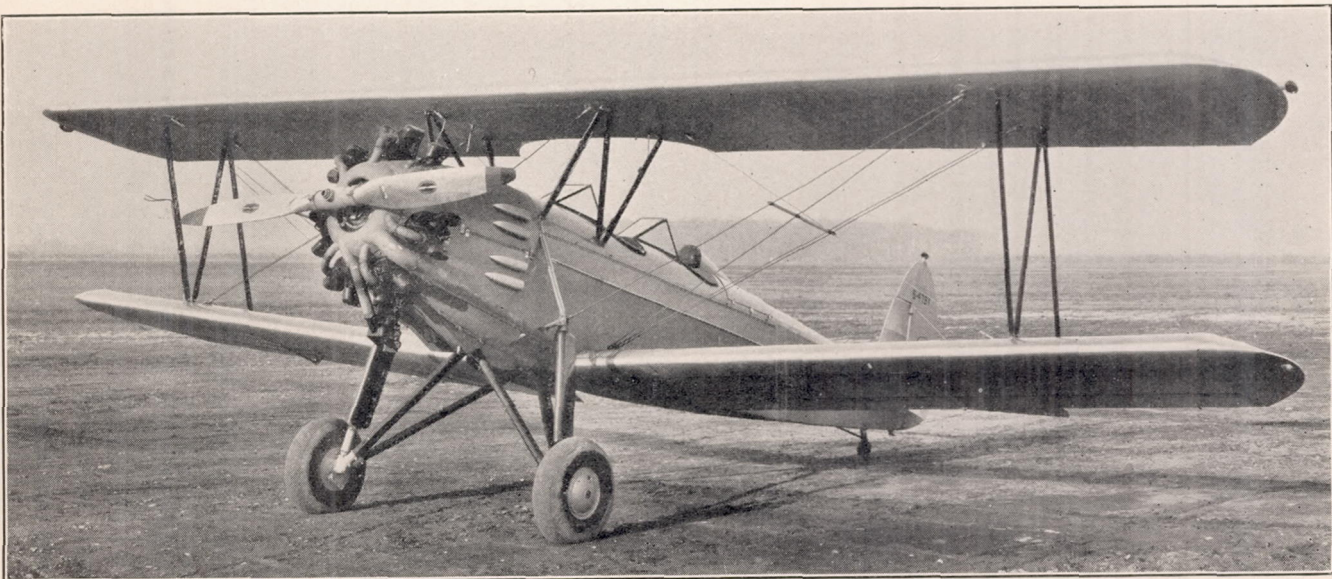
FIGURE 15.—Verville airplane with original landing gear.
