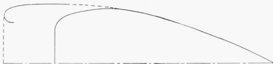
FIGURE 1.—Basic cowling shape for determining minimum drag.
