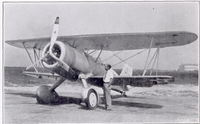
FIGURE 11.—The Curtiss BFC-1 airplane equipped with the nose-slot cowling.
