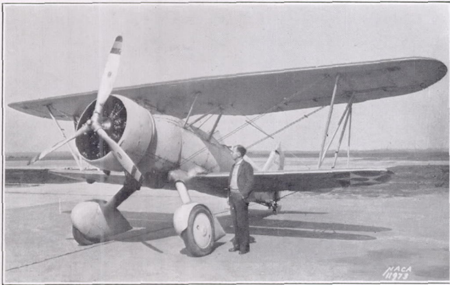
FIGURE 9.—Original cowling installation on the Curtiss BFC-1 airplane.
