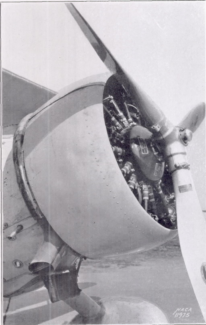
FIGURE 10.—Close-up of the original cowling on the Curtiss BFC-1 airplane
