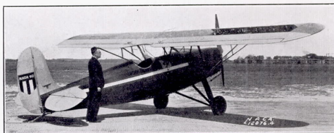
FIGURE 36.—The Fairchild 22 airplane with slot-lip ailerons as tested in flight.
