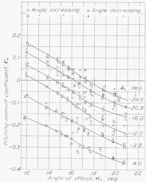
FIGURE 11.—Pitching-moment curves at different elevator angles. Fairchild 22 airplane; weight, 1,613 pounds; \delta_e , -3.6^\circ ; air speed, 56 m. p. h.
