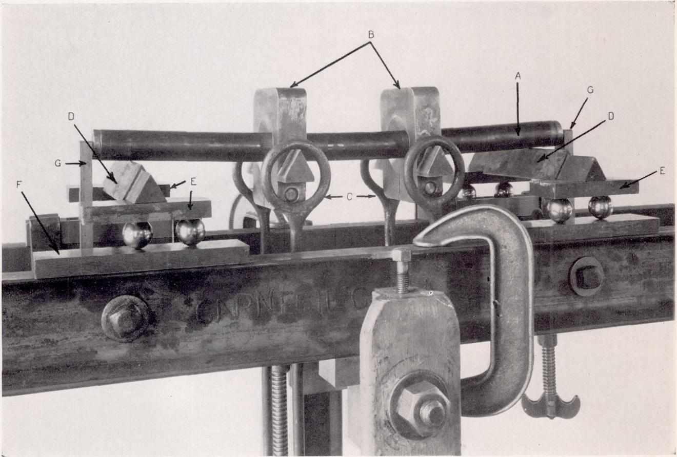
FIGURE 6.—Test to determine bending strength.
