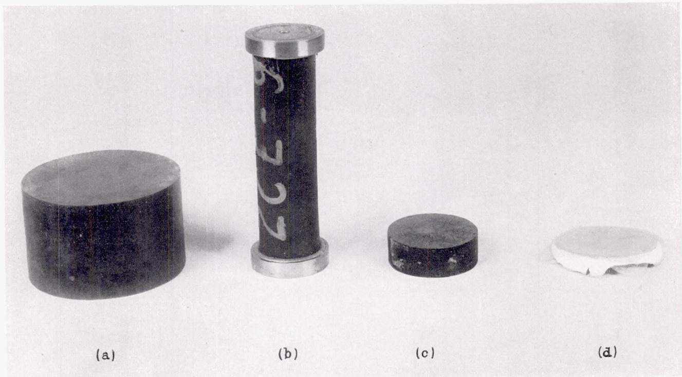
FIGURE 1.—Specimen (b), bearing blocks (a and c), and plaster chip (d).
