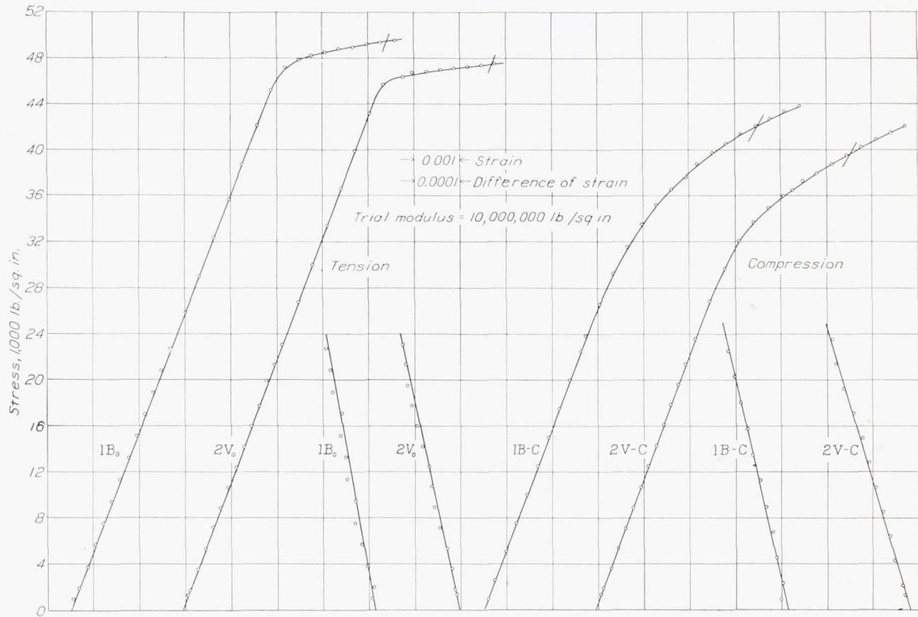
FIGURE 4.—Typical stress-strain diagrams of 17ST duralumin.
