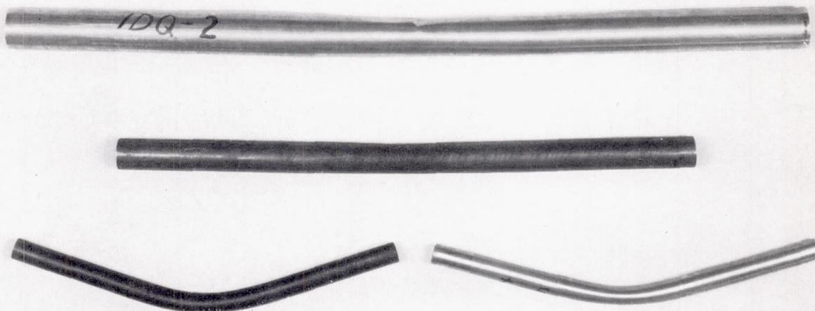
FIGURE 7.—Bending-test specimens.
