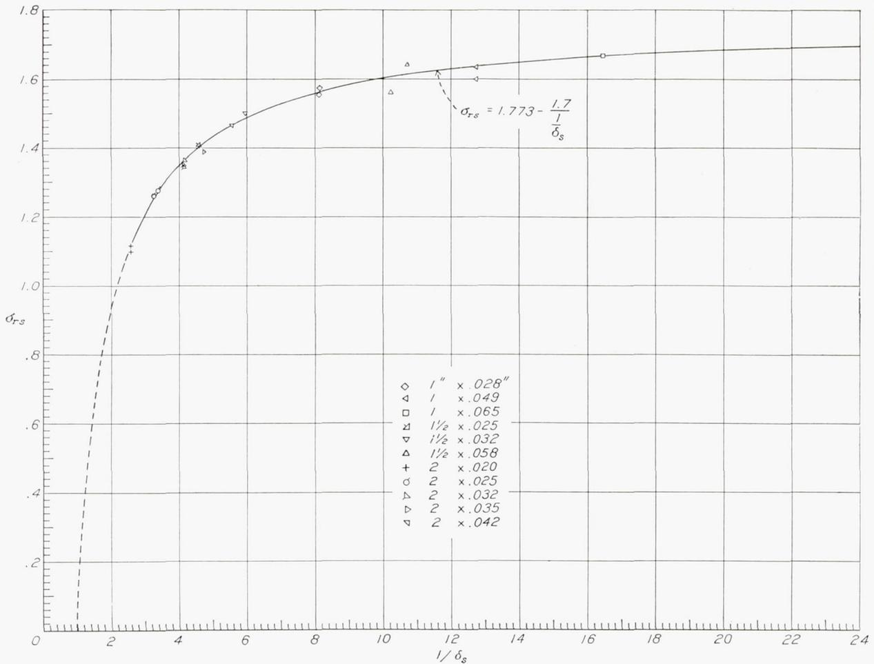
FIGURE 15.—Diagram of  $\sigma_{crs}$ ,  $1/\delta_s$  for duralumin (transverse loading).
