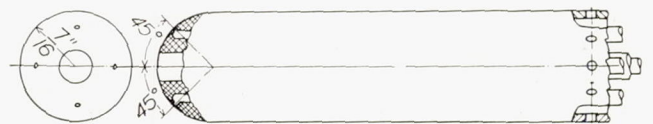
FIGURE 2.—Line drawing showing combined pitch, yaw, and pitot-static tube used for the dynamic-pressure and the downwash surveys.
