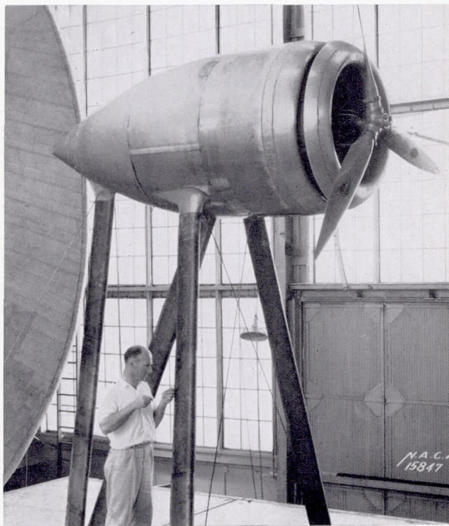
FIGURE 1.—The set-up mounted on the balance. Nose 1; slot 3; opening, 3 inches; propeller E.
