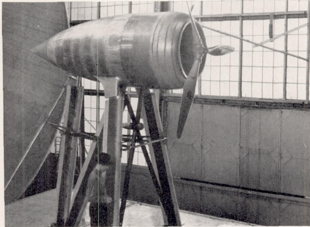
FIGURE 1.—Test set-up in tunnel. (Nose slot was closed for these tests.)
