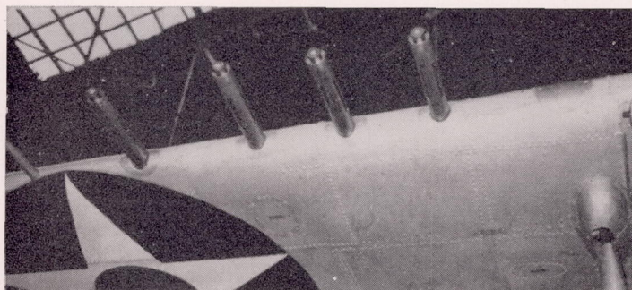
FIGURE 22.—Ten-inch barrel extension in low position on right wing. Airplane 11.
