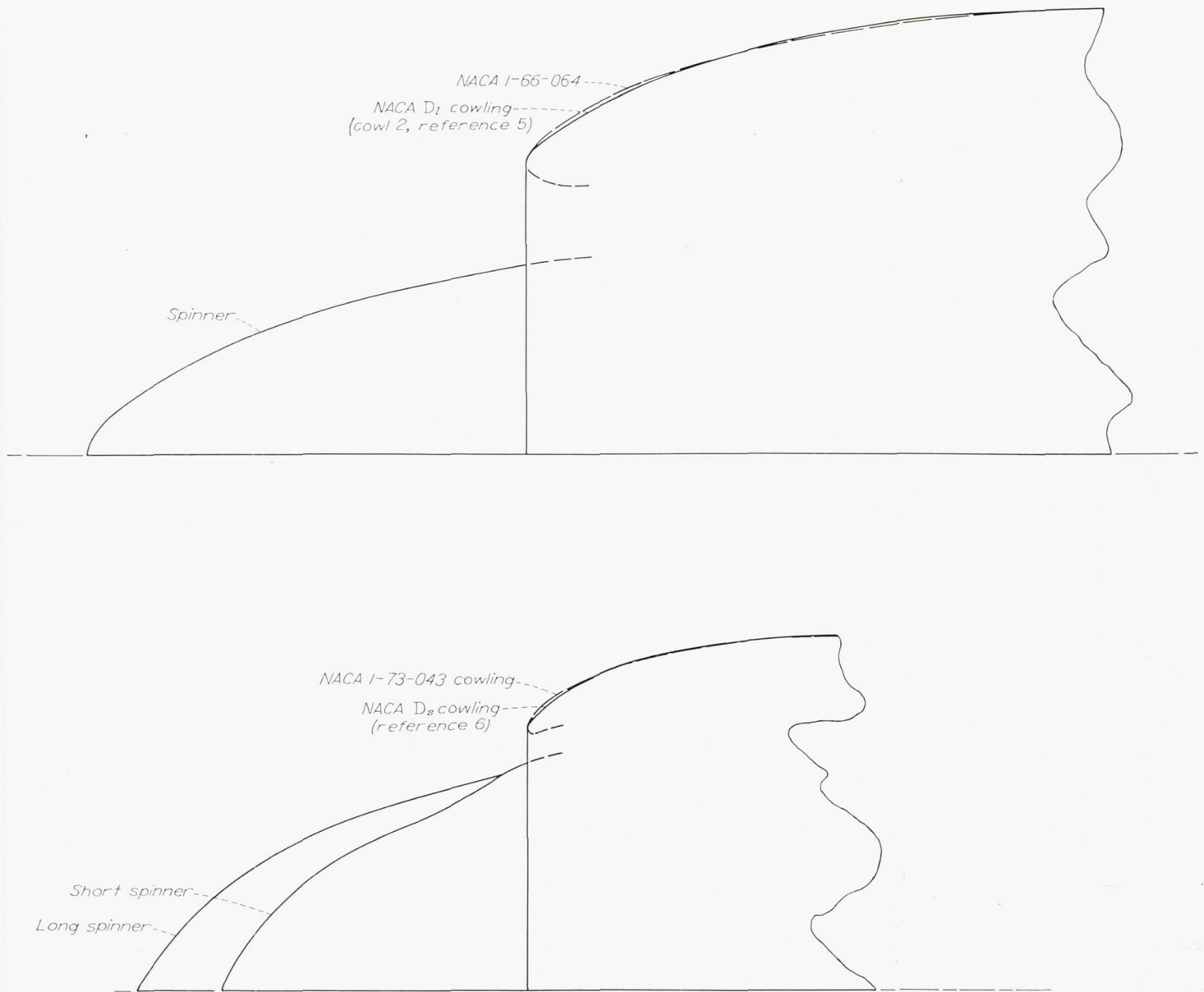
FIGURE 37.—NACA cowlings developed for use with large spinners. NACA I-series cowlings of similar proportions superimposed for comparison of profiles.
