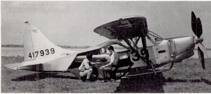
FIGURE 8.—Muffler installation, modified test airplane.
