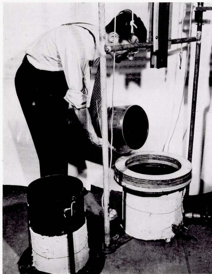
FIGURE 15.—Vacuum stretching apparatus partly disassembled after stretching a sheet of acrylic plastic. Stretched piece is on end of form which is held by operator.
