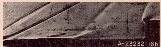
FIGURE 18.—Pure laminar and transitional separations induced by an incident shock wave; M_o=2.4 .
