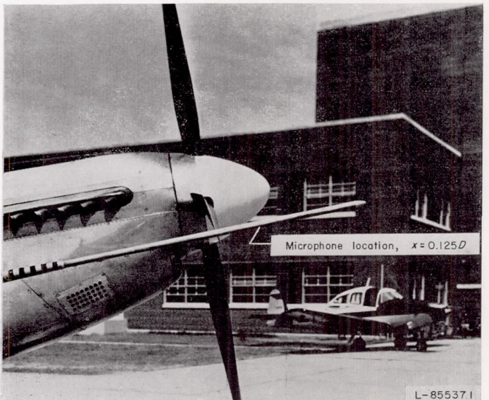
FIGURE 3.—Three microphone locations used on the test airplane during the investigation. y = 0.655D for all positions.
