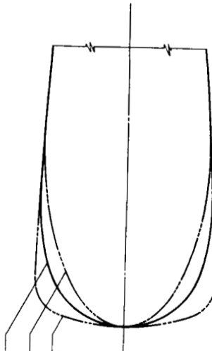
FIGURE 3c: AERODYNAMIC BALANCE NOSE SHAPES FLIGHT TESTED ON RUDDER SECTION TAKEN AT REFERENCE STATION 40
