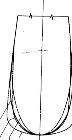
FIGURE 3b: MODEL SBD-1: REPRESENTATIVE HORIZONTAL SURFACE AIRFOIL SECTION WITH FINAL ELEVATOR BALANCE NOSE SHAPE AIRFOIL: MODIFIED N-69 WITH 12% CHORD EXTENSION AND STRAIGHT SIDED AFTERBODY, THICKNESS VARIABLE FROM 10.9% TO 7.5% ALONG SPAN ELEVATOR TRAVEL: THEORETICAL LIMIT FOR UNPORTING: \pm 24^\circ DESIGN STOPS AT 30^\circ UP, 20^\circ DOWN SECTION TAKEN AT REFERENCE STATION 46 \frac{1}{2} : CHORD = 50.83 INCHES
