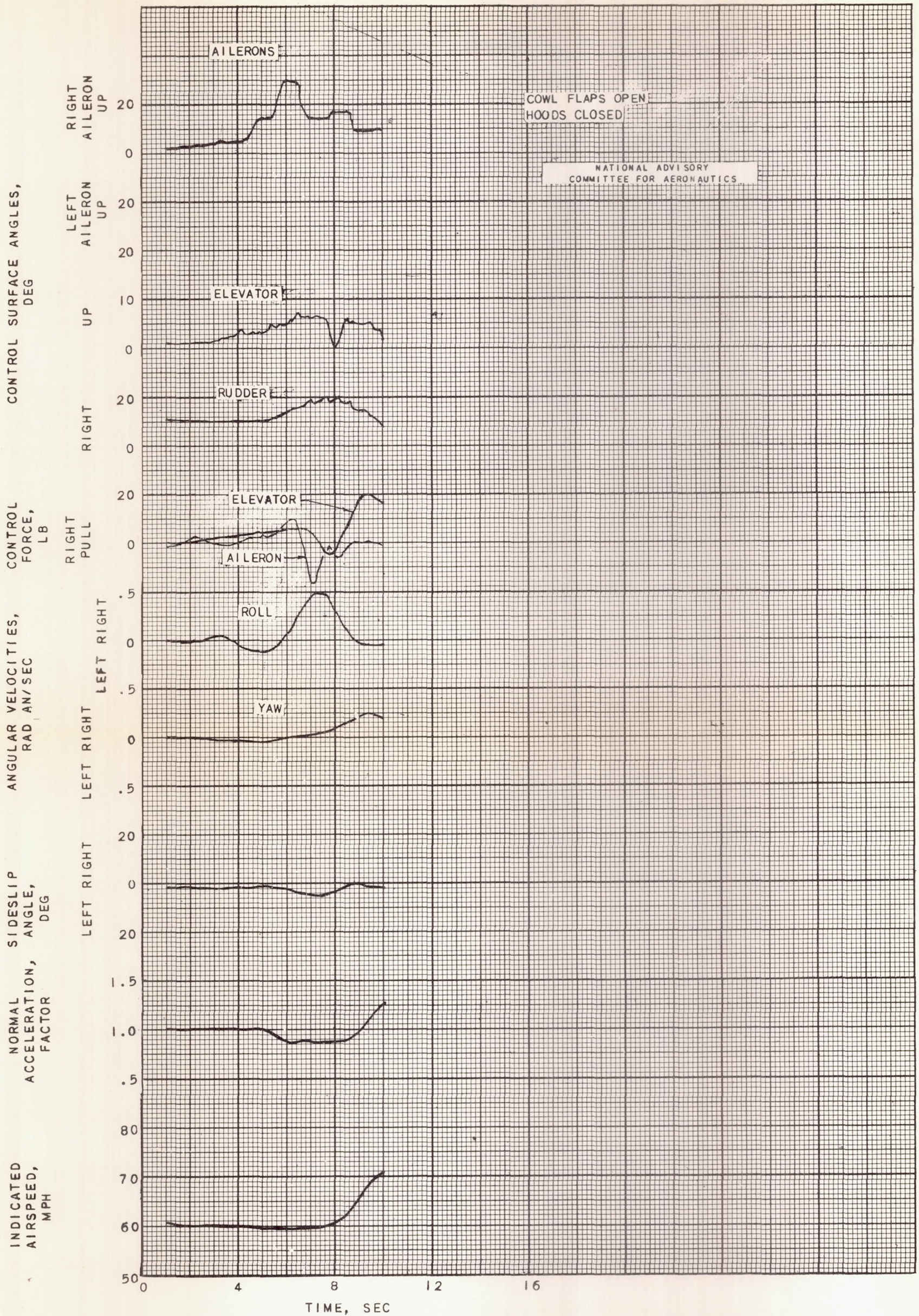
FIGURE 53. - TIME HISTORY OF A STALL, RATED POWER, FLAPS DOWN. STICK BACK TO STALL; AILERONS ALONE USED TO ATTEMPT CONTROL. RUDDER MOVED UNINTENTIONALLY.
