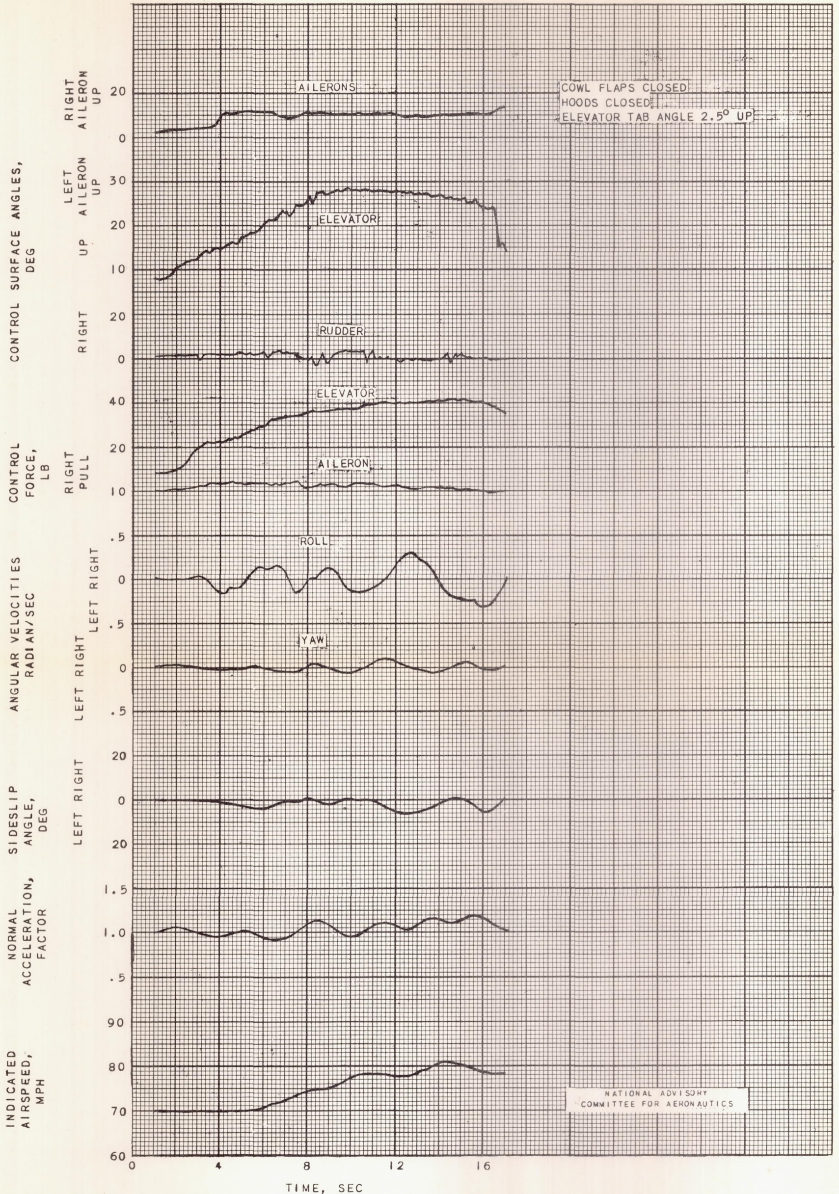
FIGURE 59. - TIME HISTORY OF A STALL, POWER OFF, FLAPS ONE-HALF DOWN. STICK BACK AND HELD WHEN STALL BECAME EVIDENT; ATTEMPT MADE TO HOLD AILERONS AND RUDDER FIXED.
