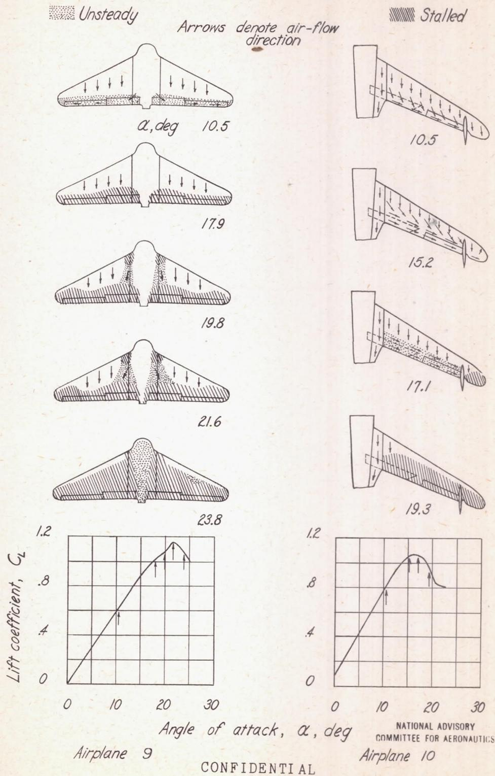
Figure 5.- Stall progressions for airplanes with swept-back wings.
