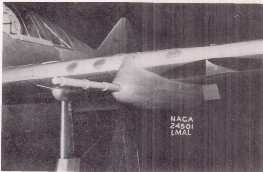
Figure 24.- Underslung-cannon installation 1.
