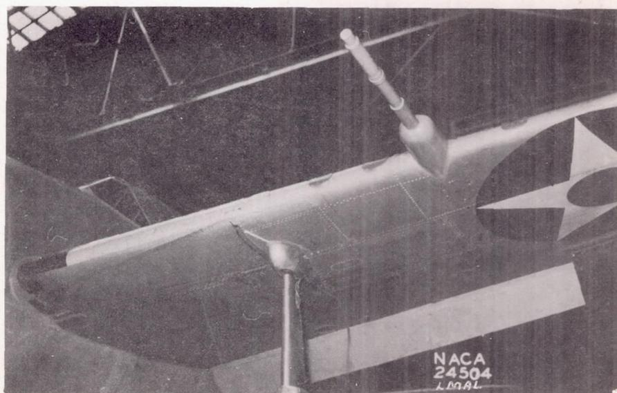
Figure 25.- Submerged-cannon installation.
