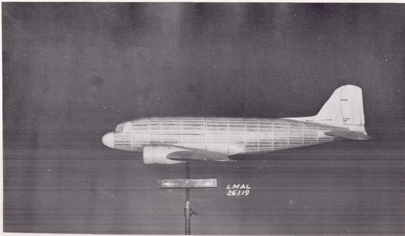
Figure 3.- Side view of the \frac{1}{23.75} -scale model of the Douglas DC-3 airplane.
