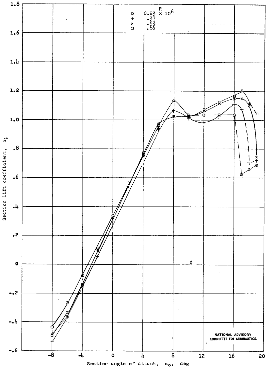
(a) Model having 6-inch chord in LTT. Figure 2.- Lift characteristics of the NACA 65 3 -418 airfoil section.
