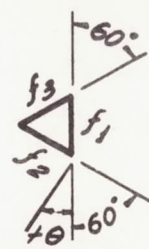
DETAIL b DELTA ROSETTE ON UPPER SURFACE & LEADING EDGE OF WING
