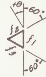
DETAIL c DELTA ROSETTE ON LOWER SURFACE OF WING
