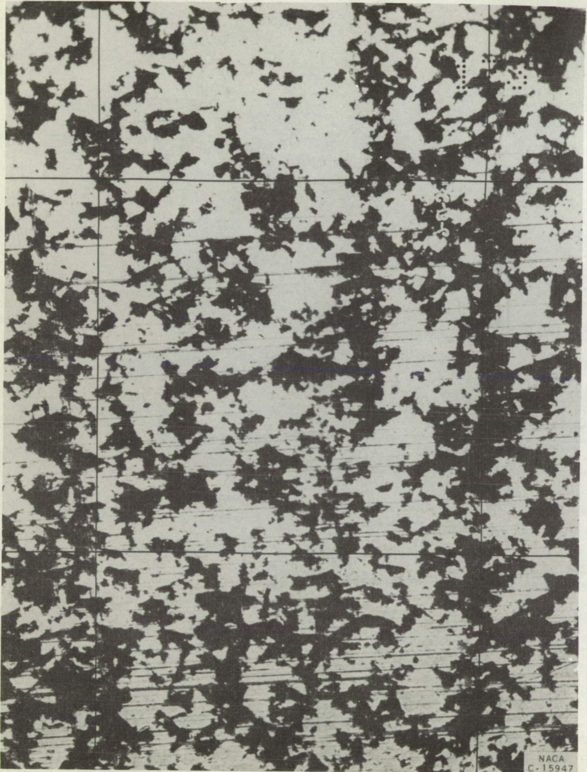
Figure 24.- Plan view of porous chromium-plated cylinder in ring travel, after test. Porosity, 40 percent. X100.
