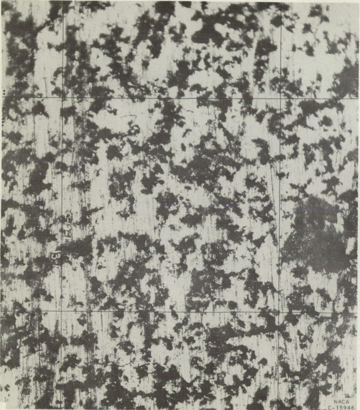
Figure 23.- Plan view of porous chromium-plated cylinder above ring travel; after test. Porosity 52 percent. X100
