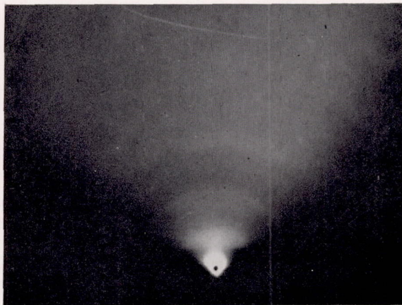
Figure 6.—Electron-diffraction pattern from a lopped cast-iron ring showing \alpha -iron plus graphite. Camera constant, 14.0. \times 2 .
