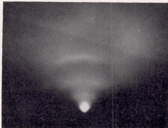
Figure 7.—Representative electron-diffraction pattern of highly oriented graphite from cast-iron ring. Test 5; camera constant, 14.0. \times 2 .
