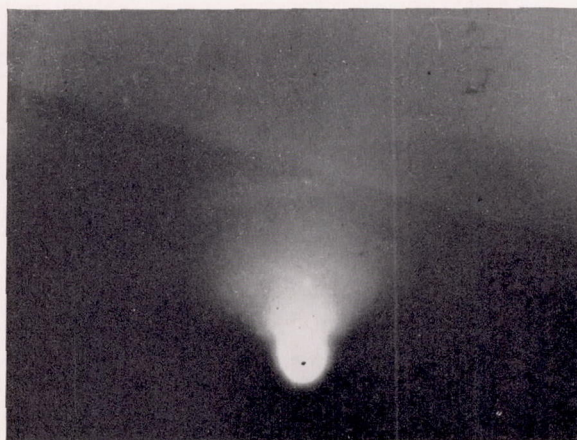
Figure 8.—Representative electron-diffraction pattern of randomly oriented graphite from cast-iron ring. Ring 3; test 3; camera constant, 14.0. \times 2 .
