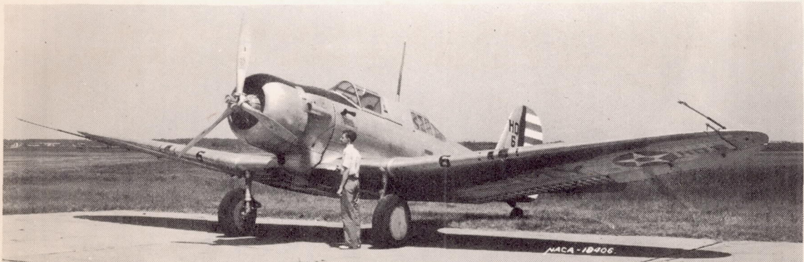
Figure 3.-One-quarter view of A-17A airplane with N.A.C.A. cowling.
