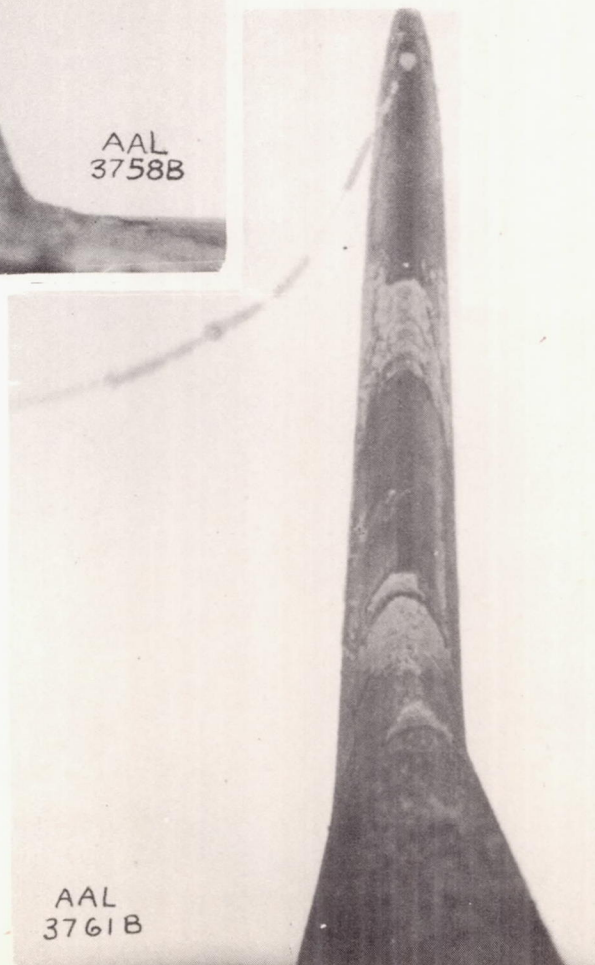
Figure 29.- The vertical stabilizer showing the accumulation of ice on the leading edge of the dorsal forward of the heated double skin, on the leading edge at the junction of the dorsal and fin, at the fin tip, and aft of the leading edge during tests 4 and 5.
