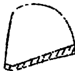
Figure 11.- Asymmetrical float for twin-float seaplane, section at step.
