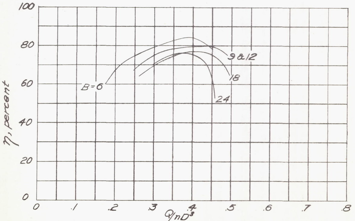
Figure 25.- Efficiencies at various solidities. \beta, 25^\circ ; no contravanes; NACA 6412 blade section.
