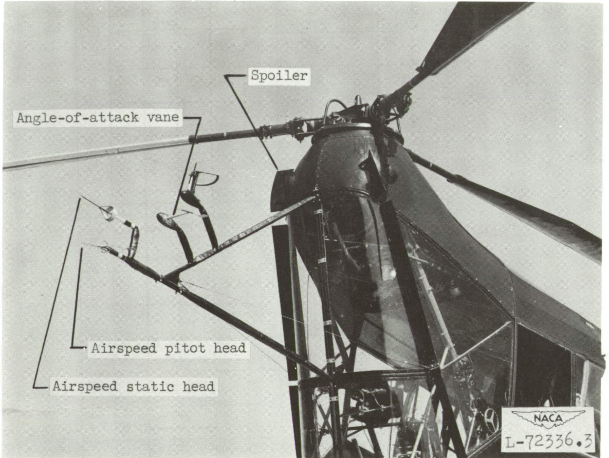
Figure 3.- Airspeed, angle of attack, and spoiler installation on test helicopter.
