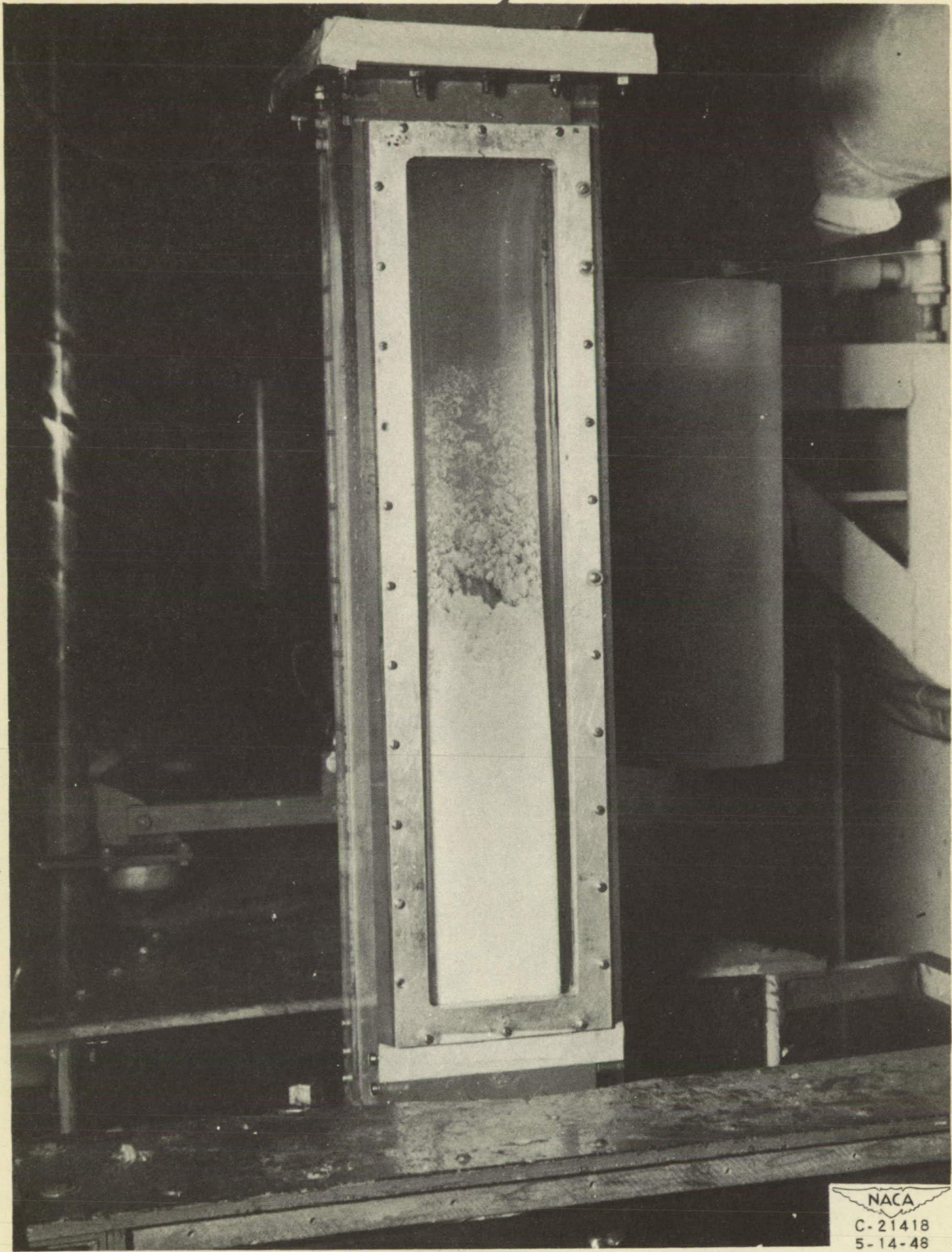
Figure 13. - Ice formation in 3.4- by 3.4-inch tunnel. Mach number, 1.45; dew point, 70° F.
