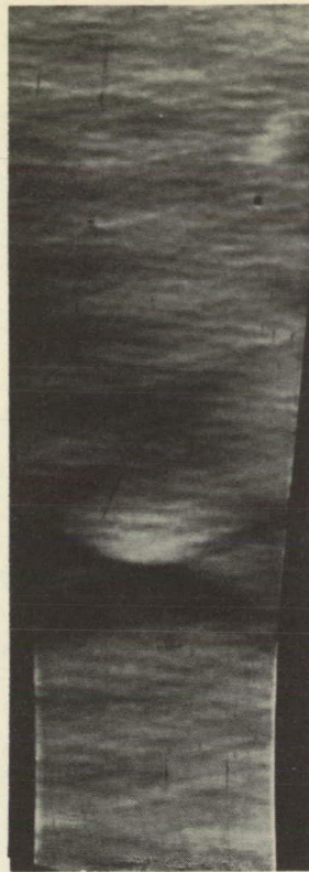
(b) Condensation shock in figure 14(a) showing change in thickness with movement downstream.
