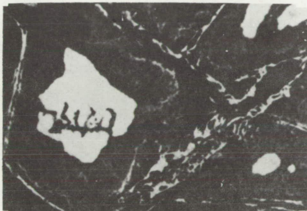
Figure 10. - Structure of oxide (iron silicate) in cast iron.
