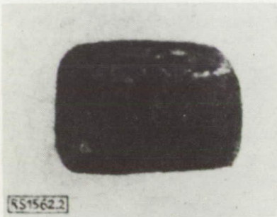
Figure 2. - Oxidized specimen of copper.
