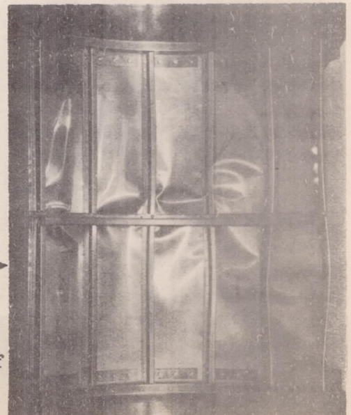
Figure 28.- Failure of panel with Z-sections under comp.
