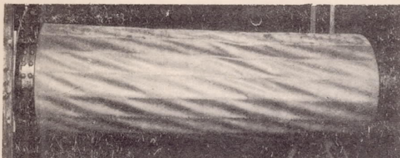
Figure 35.- Failure of full shell with Z-sections under pure twist.
