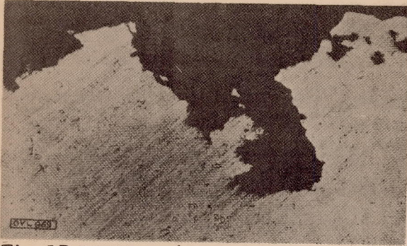
Fig.13 Pitting (deep local corrosion)
