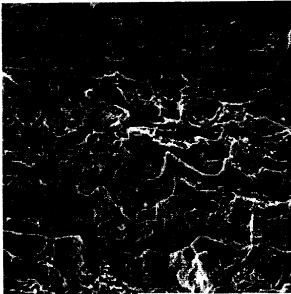
Fig. 1-8 160X. Region B. An area on the shear lip.
