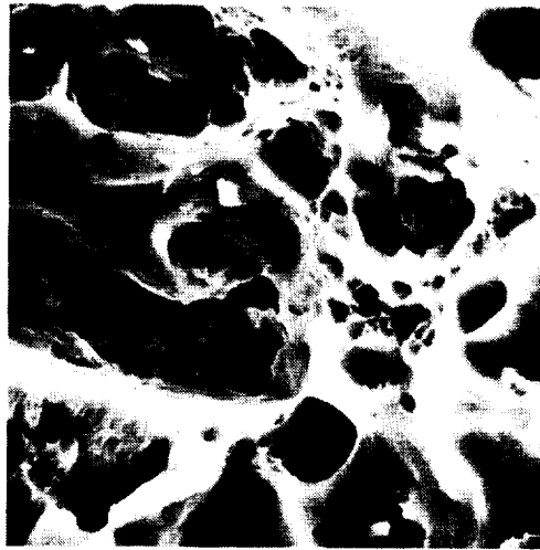
Fig 2-8 1250X Region B. Large and small dimples.
