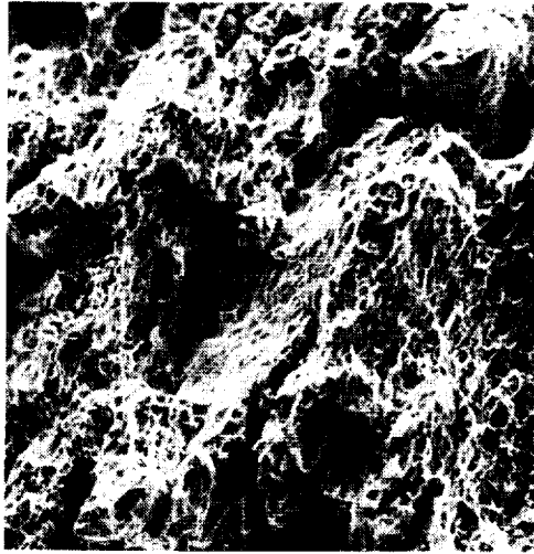
Fig 3-32 160X Region B. Region near the fracture origin.
