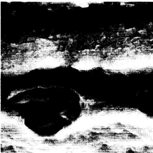
Fig. 1-15 2500X. Area A. The brittle inclusions in Fig. 1-14.
