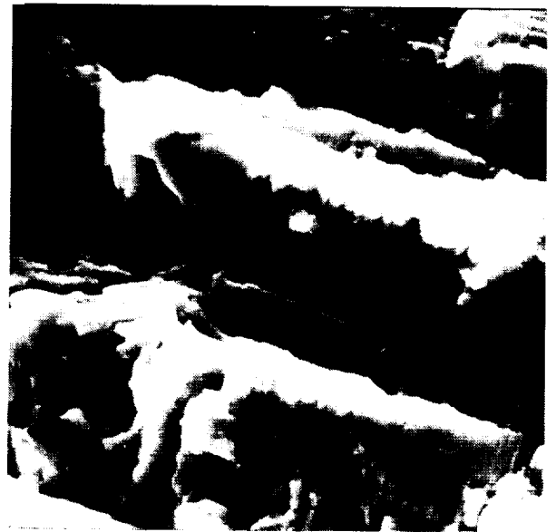
Fig. 4-51 Region 4. Fatigue striations.
