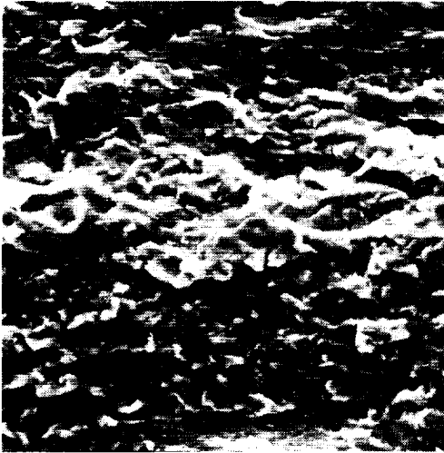
Fig. 3-40 Region 3. Fatigue striations. 640X
