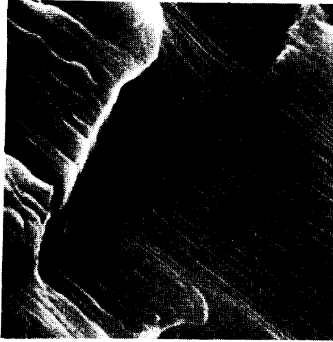
Fig. 5-42 Region 3. Fatigue striations. 640X
