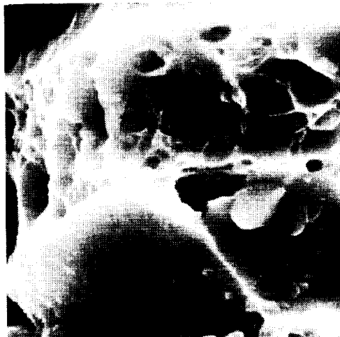
Fig. 1-22 5000X Area A. Microdimples found in the center of Fig. 1-21.
