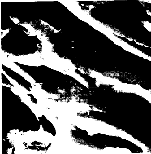
Fig. 1-36 1250X Region 2. Faint fatigue striations.
