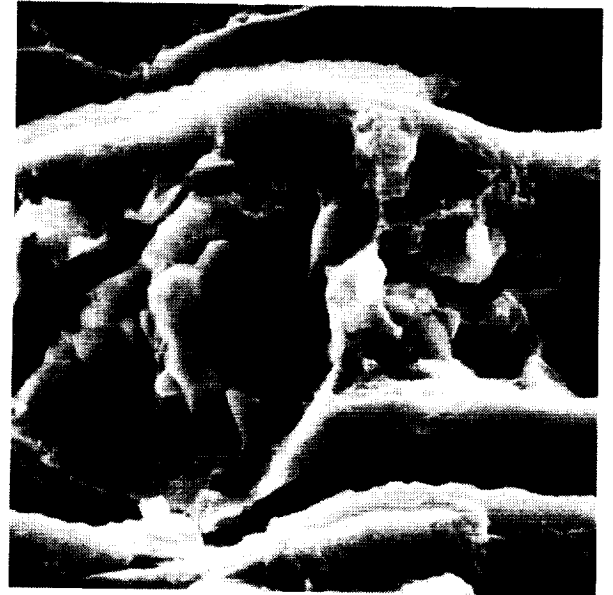
Fig. 1-30 2500X Area A. Fine dimples from Fig. 1-29.
