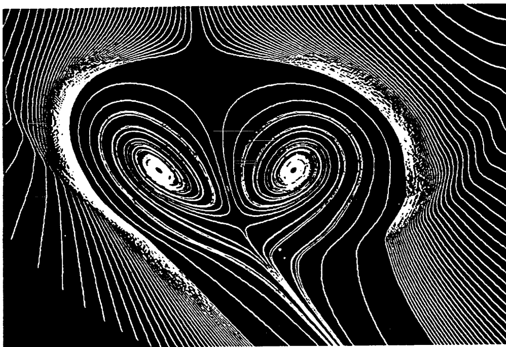
Fig. (15) - Enlarged streamline pattern showing the topology of vortex lift-off, Reduced Navier-Stokes solution, Test Case 3.2 initial conditions.
