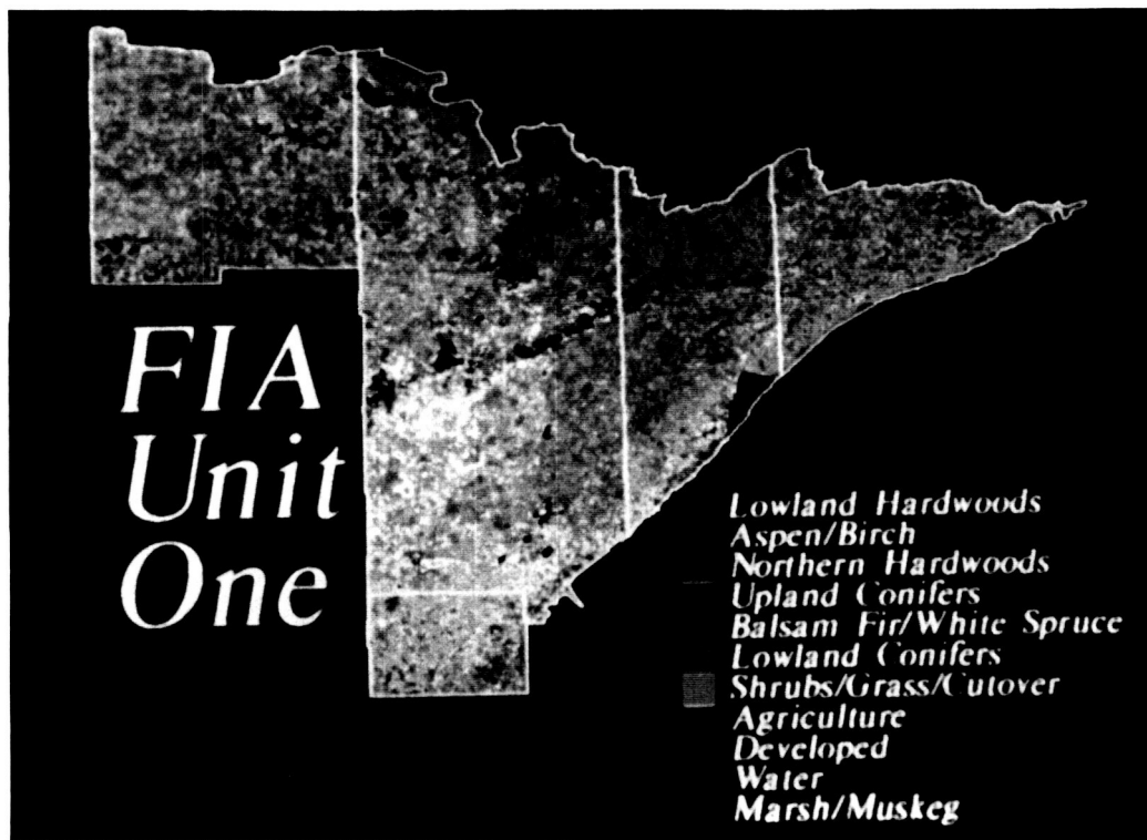
Figure 6. Final classification of Landsat TM data of entire five-county study area (FIA unit 1).
