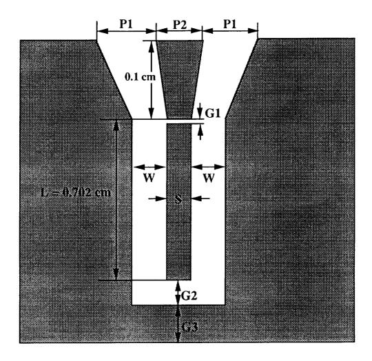
P1= 21 mils, P2 = 22 mils, W = 530  $\mu m,$  S = 200  $\mu m,$  G1 = 50  $\mu m,$  G2 = 530  $\mu m,$  G3 = 630  $\mu m$
