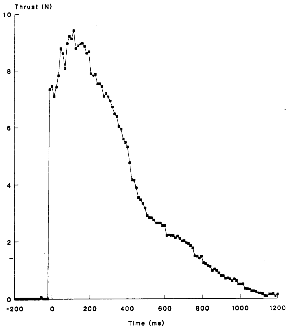
Figure 5.3: Carbon dioxide thruster with 0.1 inch nozzle
