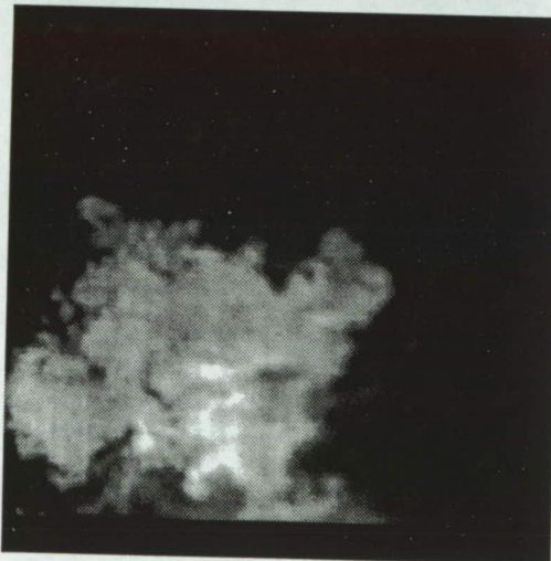
Figure 4.18. Instantaneous Rayleigh scattering images with water-seeded helium fuel at x/d_j=23.8 .
