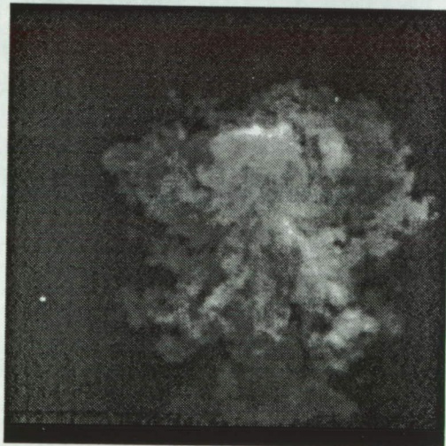
Figure 4.21. Instantaneous Rayleigh scattering images for straight case with water-seeded air fuel at twice matched pressure.
