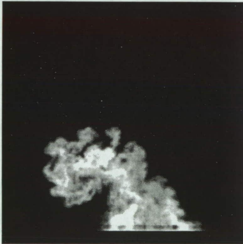
Figure 4.14. Instantaneous Rayleigh scattering images with water-seeded helium fuel at x/d_j=7.8 .
