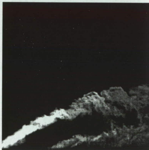
Figure 4.10. Instantaneous Rayleigh scattering images with water-seeded helium fuel at side view.
