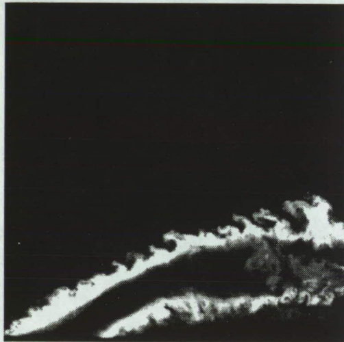
Figure 4.9. Instantaneous Rayleigh scattering images with water-seeded air fuel at side view.
