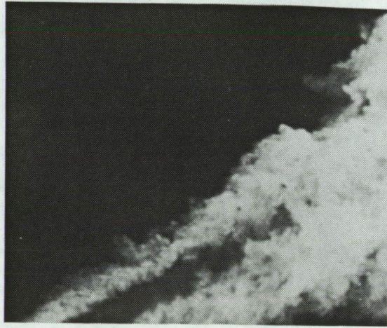
Figure 4.35. Instantaneous Rayleigh scattering image of fuel jet discharging into stagnant air with water-seeded air fuel at side view.
