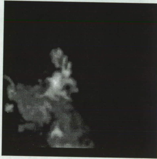
Figure 4.17. Instantaneous Rayleigh scattering images with water-seeded air fuel at x/d_j=23.8 .
