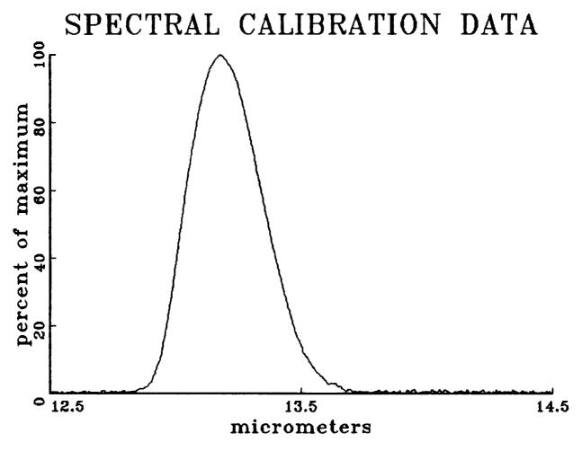
LOWER HALF FOWER POINT AT UPPER HALF POWER POINT AT PEAK POWER AT 13.023 micrometers 13.375 micrometers 13.186 micrometers
