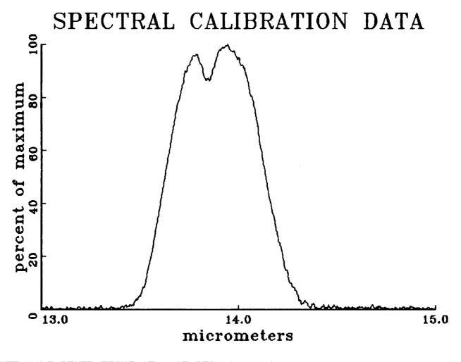
LOWER HALF FOWER POINT AT UPPER HALF FOWER POINT AT PEAK POWER AT 13.630 micrometers 14.147 micrometers 13.952 micrometers
