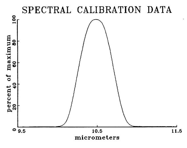
LOWER HALF FOWER FOINT AT UPPER HALF POWER FOINT AT PEAK POWER AT 10.259 micrometers 10.725 micrometers 10.498 micrometers
