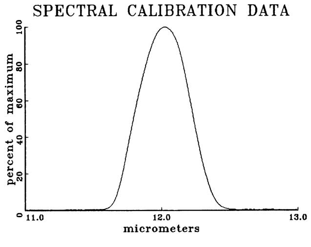
LOWER HALF POWER FOINT AT UPPER HALF POWER POINT AT PEAK POWER AT 11.799 micrometers 12.246 micrometers 12.032 micrometers
