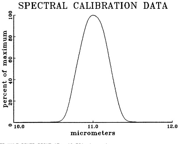
LOWER HALF POWER POINT AT UPPER HALF POWER POINT AT PEAK POWER AT 10.791 micrometers 11.239 micrometers 11.002 micrometers
