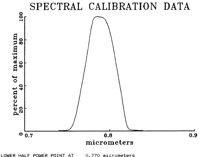
LOWER HALF POWER POINT AT UPPER HALF POWER POINT AT PEAK POWER AT 0.770 micrometers 0.810 micrometers 0.786 micrometers
