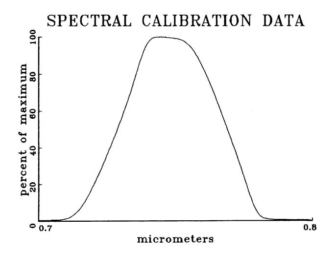
LOWER HALF POWER POINT AT UPPER HALF POWER POINT AT PEAK POWER AT 0.729 micrometers 0.769 micrometers 0.745 micrometers
