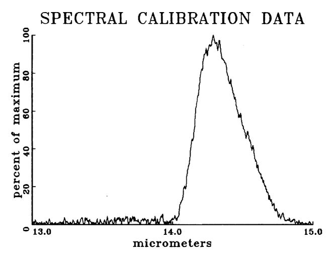
LOWER HALF POWER FOINT AT UPPER HALF POWER POINT AT PEAK POWER AT 14.163 micrometers 14.521 micrometers 14.302 micrometers
