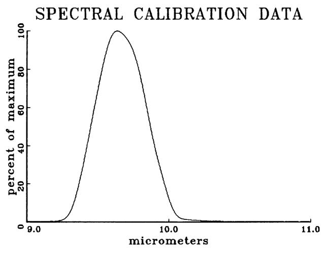
LOWER HALF POWER POINT AT UPPER HALF POWER POINT AT PEAK POWER AT 9.451 micrometers 9.877 micrometers 9.642 micrometers
