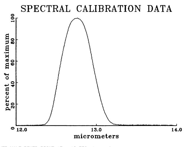
LOWER HALF POWER POINT AT UPPER HALF POWER POINT AT PEAK POWER AT 12.539 micrometers 12.986 micrometers 12.775 micrometers
