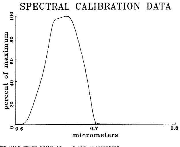
LOWER HALF POWER POINT AT UPPER HALF POWER POINT AT PEAK POWER AT 0.635 micrometers 0.688 micrometers 0.664 micrometers
