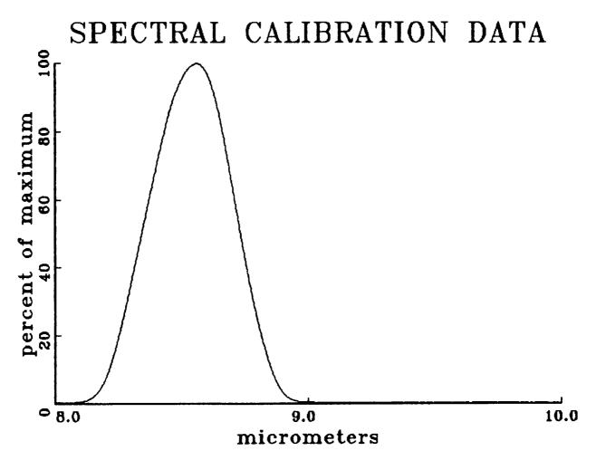
LOWER HALF POWER POINT AT UPPER HALF POWER POINT AT PEAK POWER AT 8.342 micrometers 8.738 micrometers 8.563 micrometers
