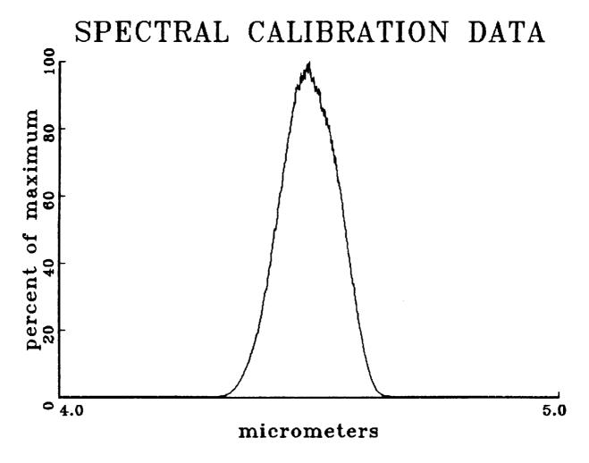
LOWER HALF POWER POINT AT UPPER HALF POWER POINT AT PEAK POWER AT 4.436 micrometers 4.578 micrometers 4.503 micrometers
