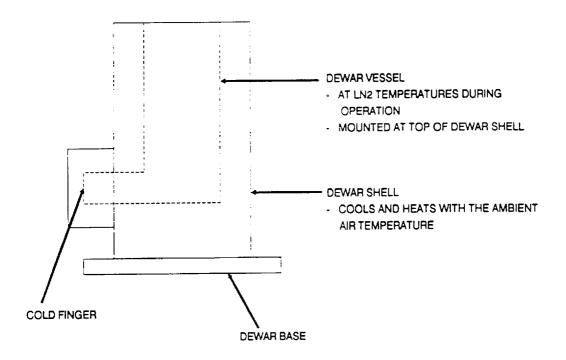
The detector arrays contained in these dewars are aligned when the dewar shell is at room temperature. As the dewar shell is cooled, thermal contraction which occurs in the shell causes the arrays to move physically closer to the dewar base.
