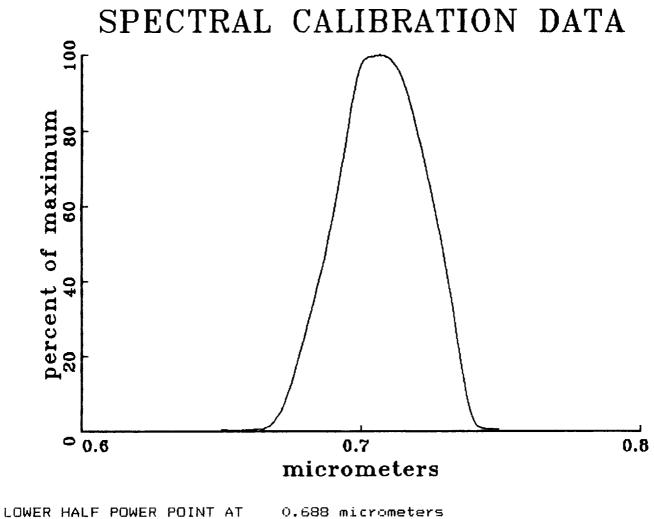
LOWER HALF POWER POINT AT UPPER HALF POWER POINT AT PEAK POWER AT 0.688 micrometers 0.729 micrometers 0.707 micrometers
