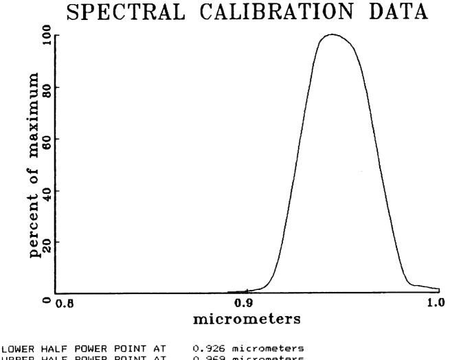
UPPER HALF POWER POINT AT PEAK POWER AT 0.926 micrometers 0.969 micrometers 0.945 micrometers
