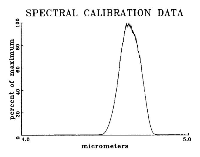
LOWER HALF POWER FOINT AT UPPER HALF POWER POINT AT PEAK POWER AT 4.582 micrometers 4.732 micrometers 4.651 micrometers
