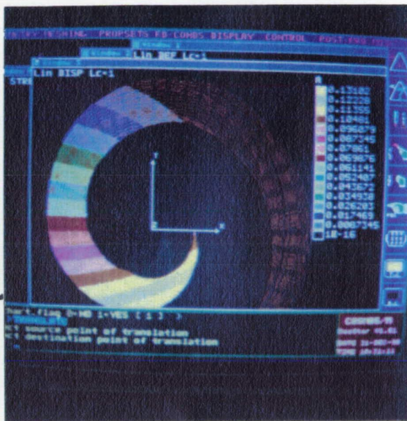
Figure 6. Single spiral leaf spring FEM: Z-axis displacement plot of SPR1.
