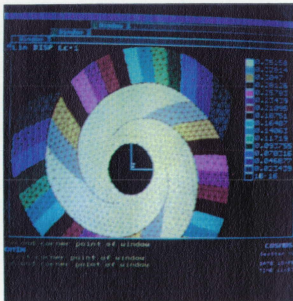
Figure 8. Z-axis displacement plot of SPR3 with 10 mm stroke @ i.d..
