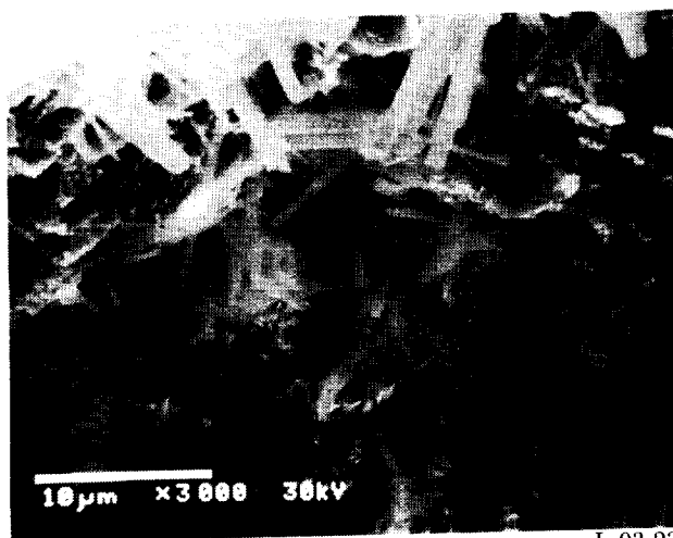
Figure 8. SEM micrograph of decomposition products along surface of \text{YBa}_2\text{Cu}_3\text{O}_{7-x} specimen stored at 100 percent relative humidity for 6 weeks.
