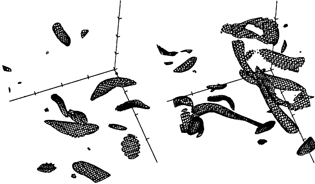
FIGURE 5. Intense vorticity isosurfaces, |\omega|/\omega' \geq 2.5 , at two different Reynolds numbers. Resolution is similar in both subsets, with the length of each axis \approx 100\eta . Left: Re_\lambda = 63 , integral scale L = 56\eta . Right: Re_\lambda = 95 , L = 80\eta . Thresholds are chosen so that worms contain about 1% of total flow volume.
