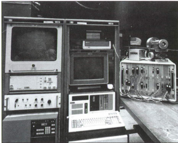
Breadboard camera and IIS (right) with a i486-based computer, additional storage, and display equipment.
