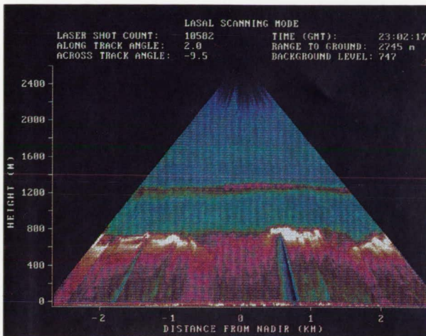
Color image of the relative backscatter intensity received by the LASAL instrument for one scanning sequence. The top of the PBL can be seen at about 800 meters.
