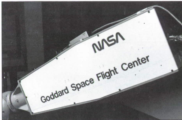
A capaciflector sensor used by a robot in the lab. This sensor could routinely detect a human or an aluminum-truss element within 1 ft of the robot.
