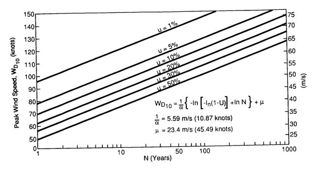
Figure 2-7. Facility design wind,  $W_{D 10}$ , with respect to the 10-m reference level peak wind speed for various lifetimes (N), KSC.
