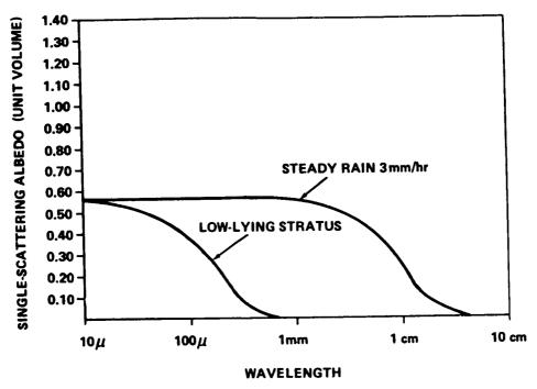
Figure 8.2 Single scattering albedo for two cloud models.
