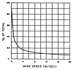
B. Correction (fw) for wind speed to the surface temperature difference (obtained from graph A). Valid only for a pressure of one atmosphere.
