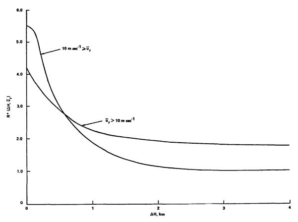
Figure 2-21. The function  $R^*$  versus  $\Delta H$  for various categories of wind speed  $\overline{u}_t$  at the reference level.
