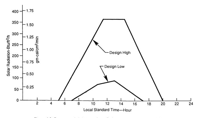
Figure 4.3 Recommended design solar radiation at ground level (ref. 4.9).
