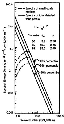
Figure 2-29. Spectra of detailed wind profiles.
