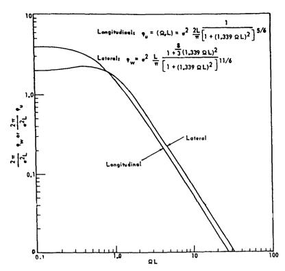
Figure 2-39. The nondimensional longitudinal and lateral,  $2\pi\Phi_w/\sigma^2L$  and  $2\pi\Phi_w/\sigma^2L$ , spectra as functions of the dimensionless frequency  $L\Omega$ .
