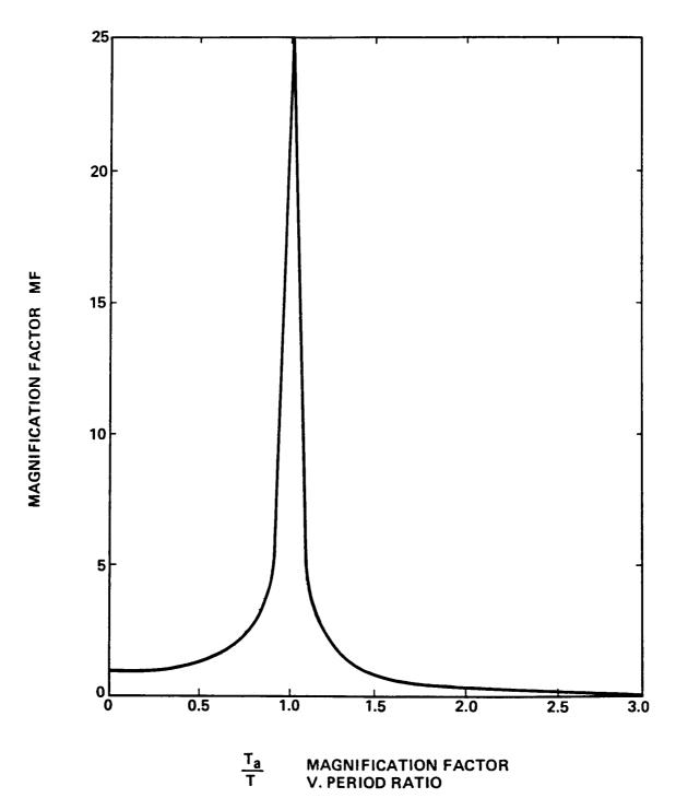
Figure 13.18 Magnification factor versus period ratio.
