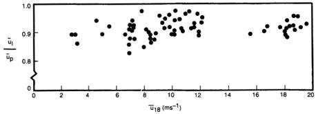
Figure 2-2A. The ratio  $\overline{u}_l / \overline{u}_P$  as a function of the 18.3-m level mean wind speed ( $\overline{u}_{18}$ ) for a 10-min sampling period.
