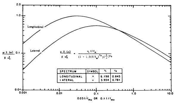
Figure 2-6.  $\omega S(\omega)/\beta u^2$  versus  $0.03f/f_m$  (longitudinal) and  $0.1f/f_m$  (lateral) for strong wind conditions.
