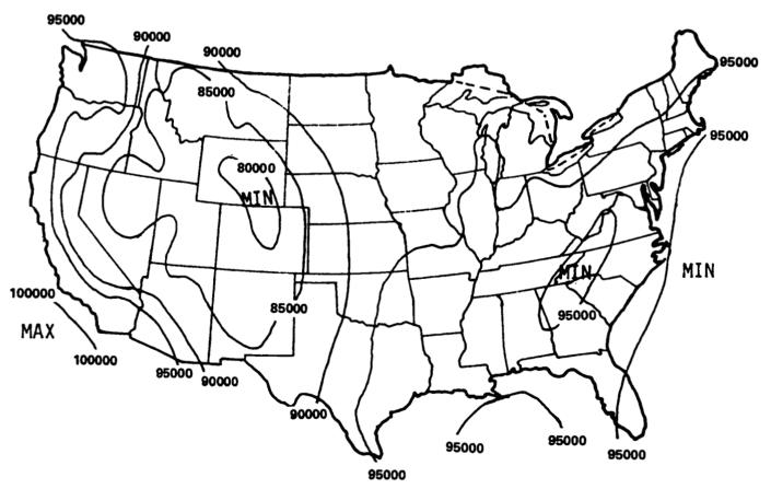
Figure 5.9 Maximum absolute station pressure (N/m<sup>2</sup>).
