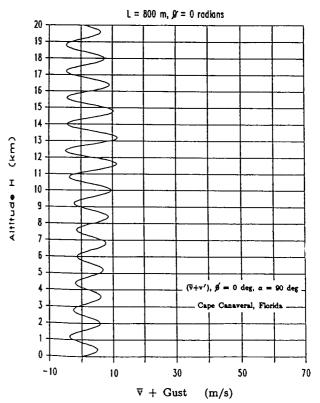
Figure 2-28. Mean meridional wind component combined with gust.
