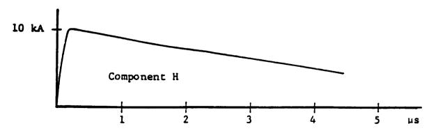
Figure 9.8 The SAE 1987 current test waveforms for severe direct lightning strikes to aircraft (ref. 9.5) (continued).
