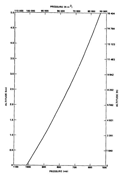
Figure 3.1 Pressure change with altitude for packaging materials (ref. 3.1).
