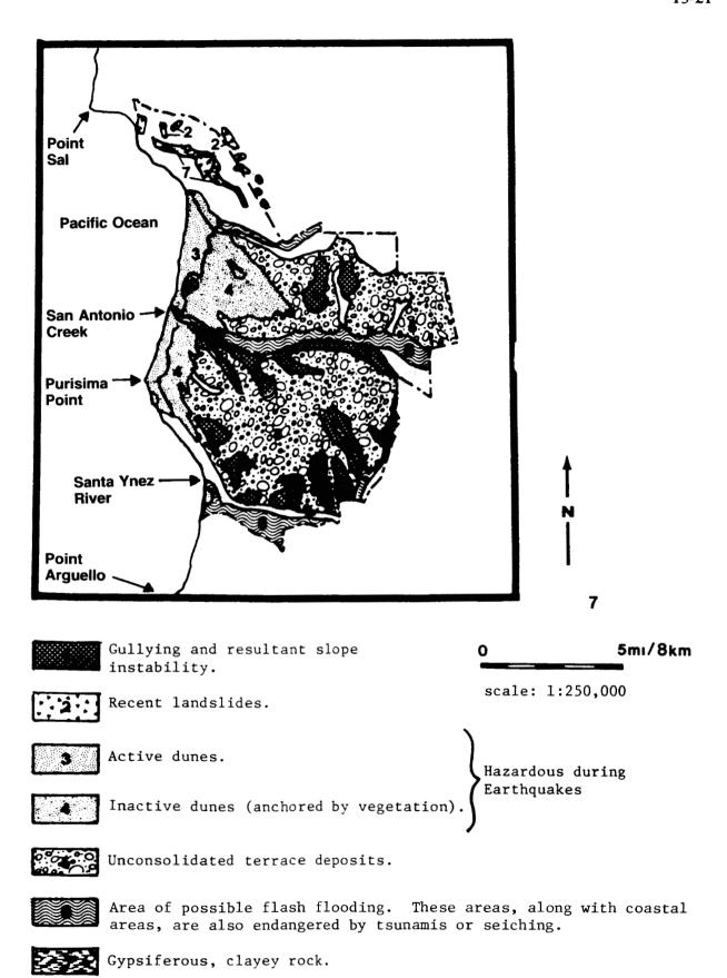
Figure 13.13 Geologic hazards of Vandenberg AFB, California.
