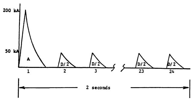
Figure 9.10 Multiple stroke lightning current test waveform consisting of a first stroke (component A) and followed by 23 subsequent strokes (attenuated D components) (ref. 9.5).
