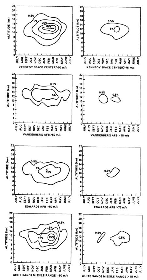
Figure 2-44. Frequency of scalar wind speed exceeding given wind speed as a function of altitude for stations indicated.
