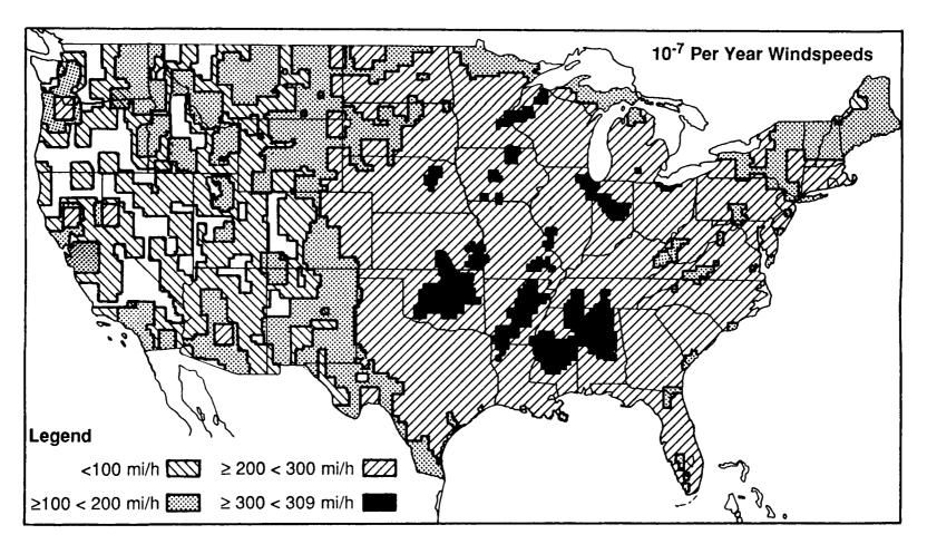
Figure 12.2 Distribution of the maximum windspeeds of tornadoes expected to occur with a 10<sup>-7</sup> or 1/10,000,000 per year probability which is required for protecting nuclear power plants in the United States (ref. 12.2).
