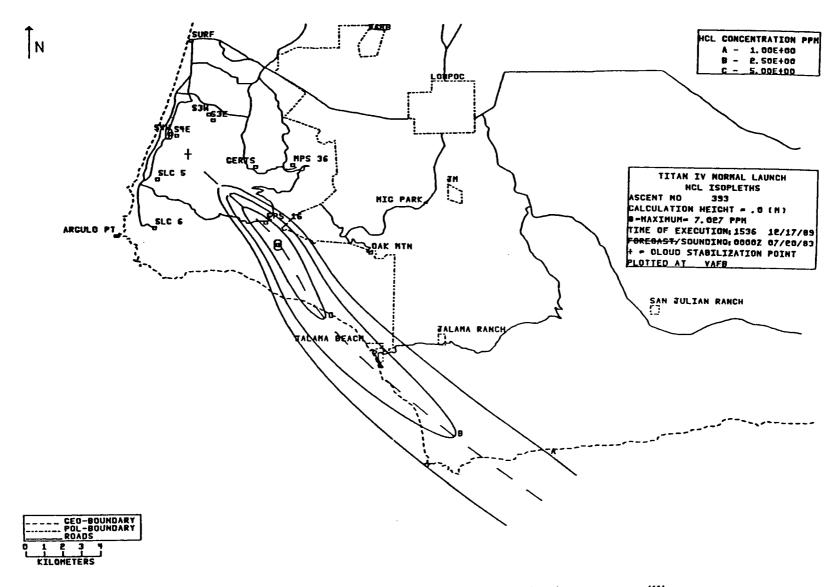
Figure 11-3. Example REEDM plot of peak HCl concentration in parts per million for a space shuttle launch.
