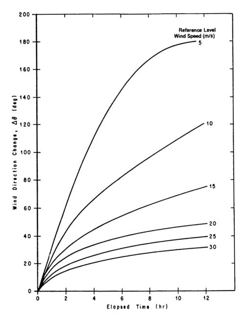
Figure 2-12. Idealized 99-percent wind direction change as a function of time and wind speed in the 150-m to 2-km altitude region of KSC.
