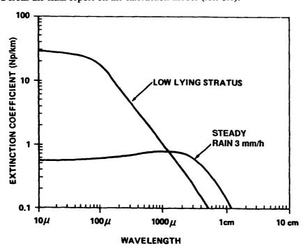
Figure 8.1 Extinction coefficient as a function of wavelength.
