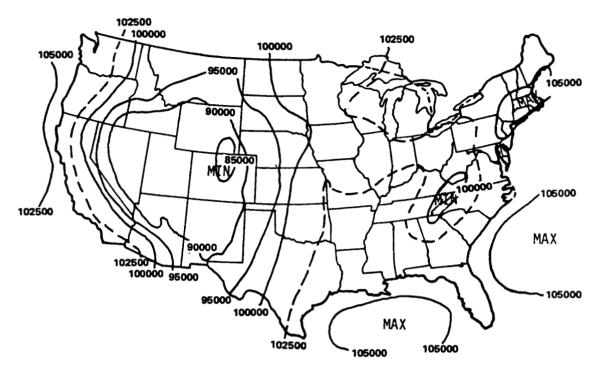
Figure 5.8 Maximum absolute station pressure (N/m<sup>2</sup>).
