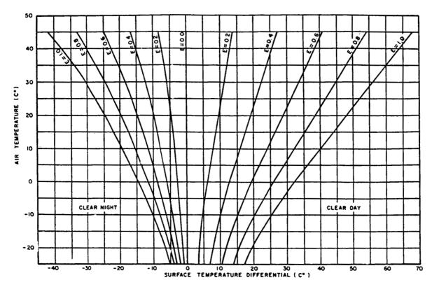
A. Surface temperature differential ( $\Delta T_{BS}$ ) with respect to air temperature for surface with emittance between 0.0 and 1.0 for a calm wind. The temperature difference, after correction for wind speed, is added or subtracted to the air temperature to give the surface (skin) temperature. Wind speed has a great effect, not because it changes the radiation part of the heat transfer, but because it makes the convective heat transfer very significant.
