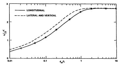
Figure 2-42. Nondimensional discrete gust magnitude,  $V_m/\sigma$ , as a function of nondimensional gust half-width.
