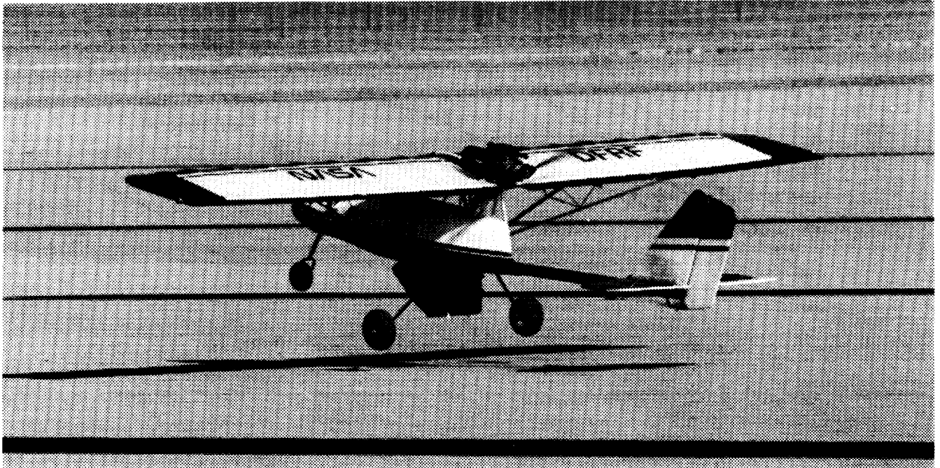
Figure 9. Spacewedge attached to the ultralight remotely piloted airplane.
