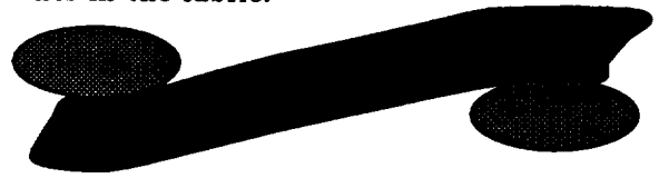
Illustration of Crimp in a Woven Fabric
