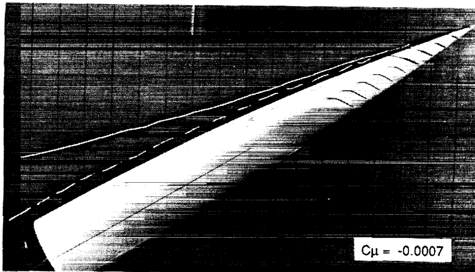
Figure 15 - Effect of Jet Blowing (Aft, Left Side, Forebody Model # 1) Circular Nozzle, 0.102 cm i.d., \alpha = 30^\circ
